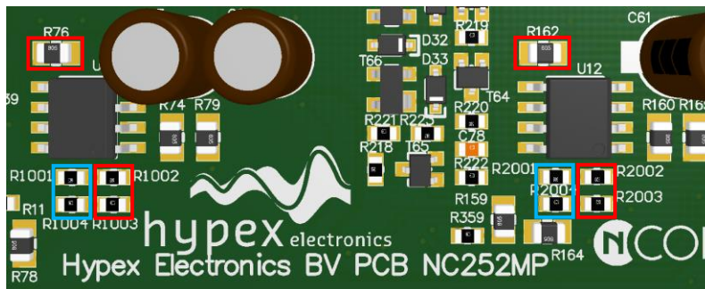
Figure 2 Resistors in the red squares need to be removed, resistors in the blue squares need to be added for unbuffered operation
